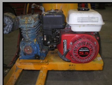
Serviced Honda Engine and Compressor
