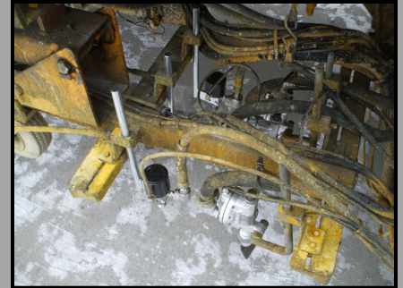
4 - KC-700 Airless Paint Guns 4 - KC-600 Bead Guns
