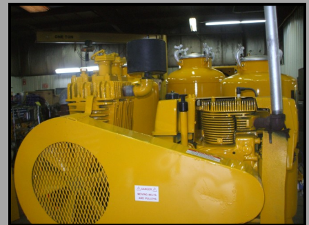
Serviced Kohler Engine and Quincy Compressor
