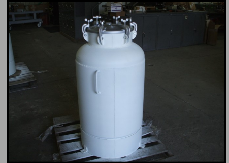
60 gallon carbon steel tank 720# bead tank
