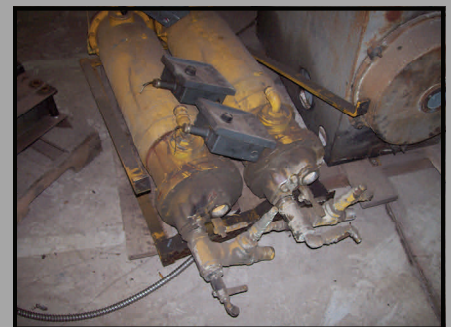
Two each 8" X 36" Basco four pass heat exchangers, stainless steel tube with cast iron bonnets
