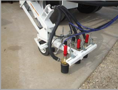
Rugged gun carriage with pneumatic lift
