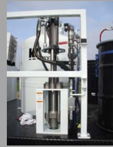
Hydraulic powered airless paint pumps
