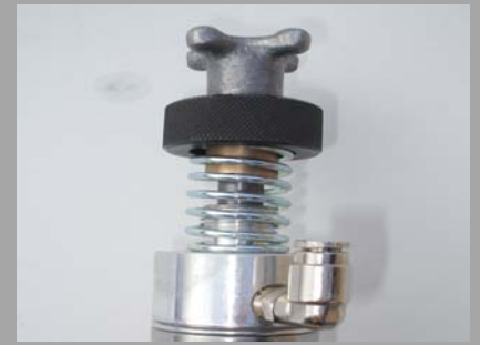
Bead flow adjustment, no tools required
