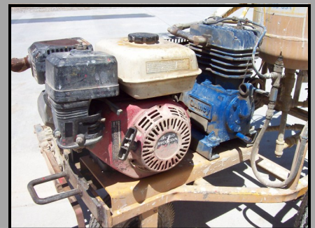
Honda 5.5 HP engine and 13.1 CFM compressor
