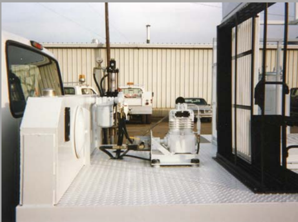
Optional compressed air system for reflective bead, air wand
