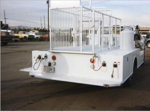
Stencil rack, paint, bead & compressed air hose reels
