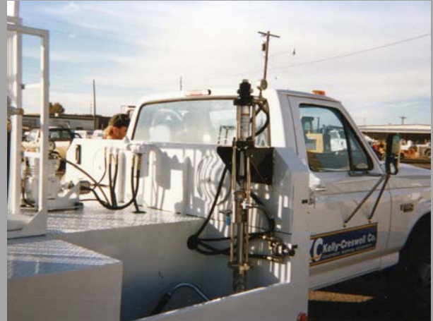
Airless paint pump(s) draw paint from 5 gal pails or optional tanks
